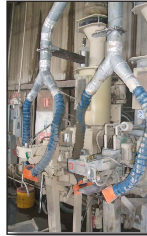
flex-loc line pickup points for bagging machines which connect to the CP-305.
