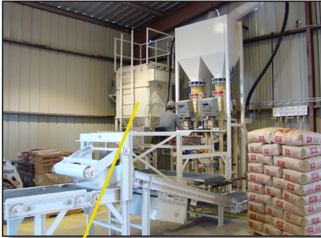
CP-305C with 55 gallon barrel drop and 6" Easy-UP ducting.
